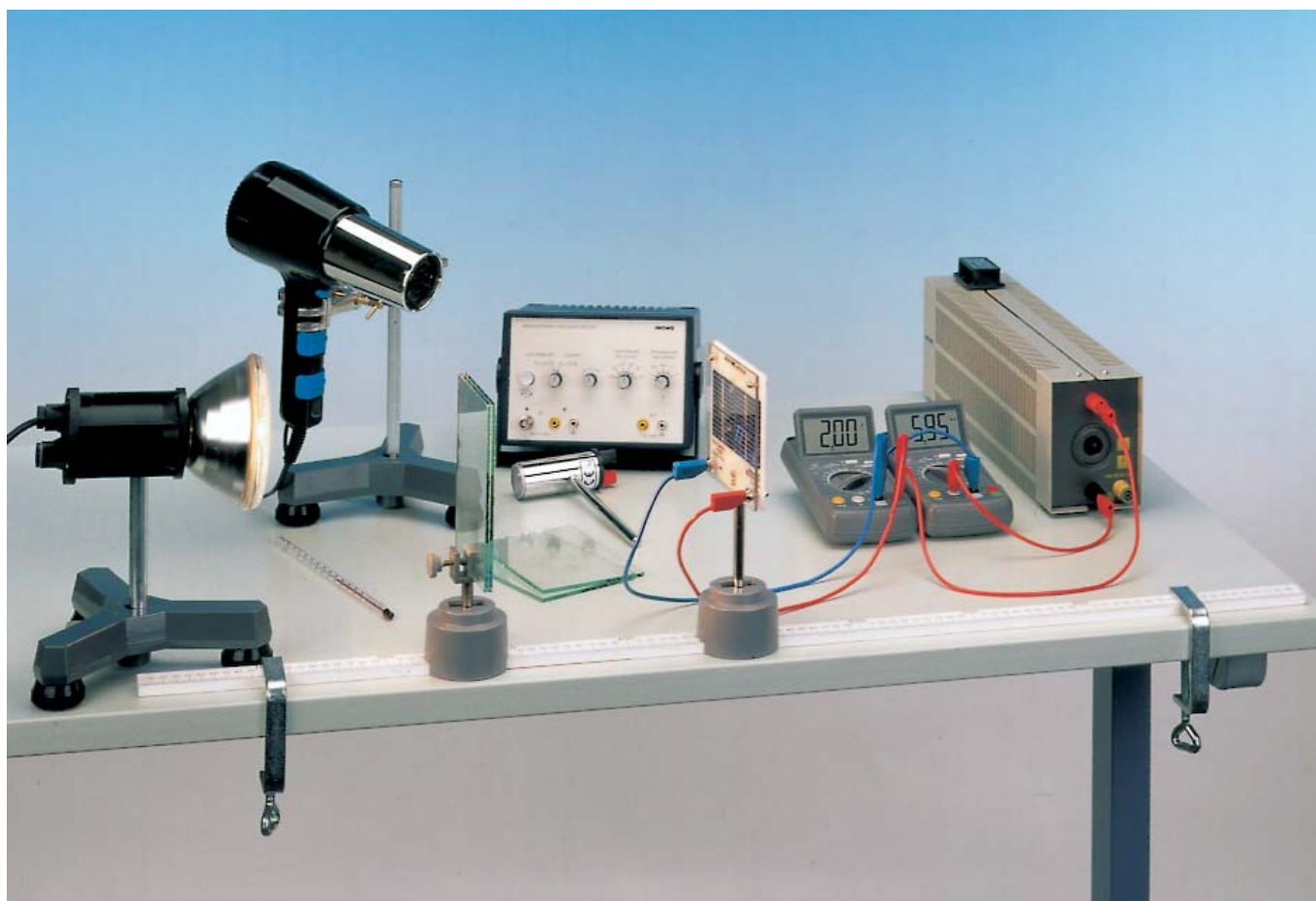
Fig. 1: Experimental set-up for determining characteristic curves.
